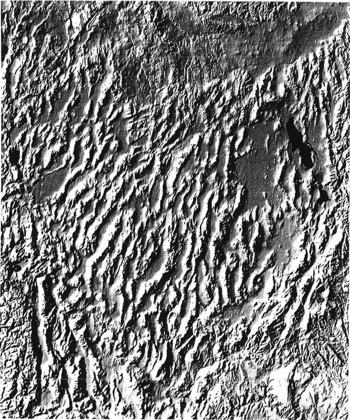
Figure 9-11. Topography of the Basin and Range Province, western United States, part of a shaded-relief image prepared by Thelin and Pike (1991) by digitizing elevation values at intervals of 805 m and illuminating the resulting digital elevation model from the west-northwest, 25° above the horizon. North is approximately toward the top of page. Vertical exaggeration 2×. Black area at upper right is Great Salt Lake; flat area farther north is Snake River Plain (cf. Fig. 9-12). Basin and Range Province extends from Wasatch fault, east of Great Salt Lake, to eastern front of Sierra Nevada (lower left corner). Albers Equal-Area Conic Projection.
